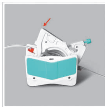
3. Press the cartridge to make the cartridge enter the working position.
